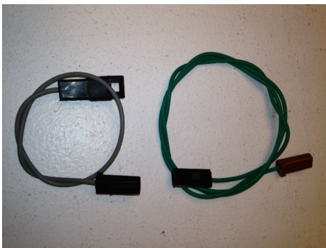
1956 LIGHTING SWITCH EXTENSION WIRES
